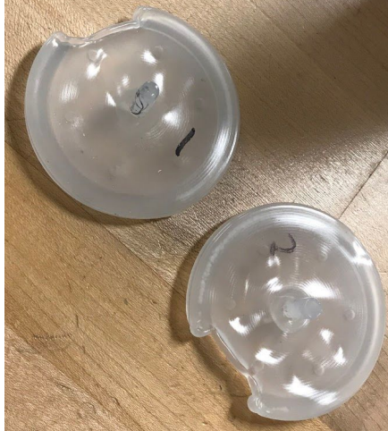
Figure 11: Attempts #1 and #2 at injection molding. Short shot and dishing occurred in both of these parts, due to shot size being too small (1.50in), and ejector pins that were too long (5.375”).
