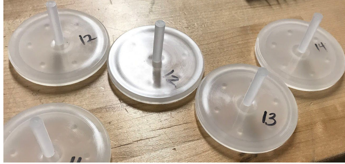
Figure 16: #12 - #15. Increased injection pressure profile from 1299 psi - 1650 psi to 1650 psi - 1800 psi. Ran this configuration four times to allow the machine to “catch-up.” Weldline and flashing still present.
