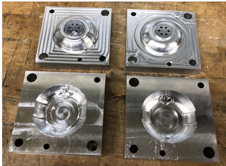
Figure 6: Two attempts at the yellow face mold. Our first attempt on the left has order of operation errors on the core and toolpath errors on the cavity. Our
