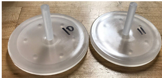
Figure 15: #10 & #11. Increased injection boost pressure to 2300 psi, and reset the injection speed profile. No more burn, but weldline still present.
