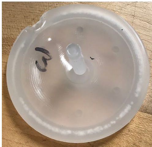
Figure 12: Attempt #3. Increased shot size to 1.75in, and shortened ejector pins. There's less dishing now, but still short shot in the far side (from the mold) of the part
