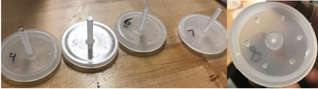
Figure 13: Attempts #4 - #8. Changes are just gradual increases in shot size up to 2.30in, and moving the injection boost pressure up to 1800 psi. There is a weldline that still exists at the far side of the part, but since flashing has occurred, we figured the next change must not have to do with the shot size.
