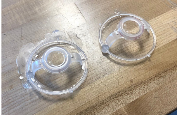
Figure 20: Attempts at injection molding the goggle. Major flashing occurring in the 2nd iteration (left, 1.25 in shot size). Excess plastic removed from 1st iteration (right, 1.50 in shot size)
